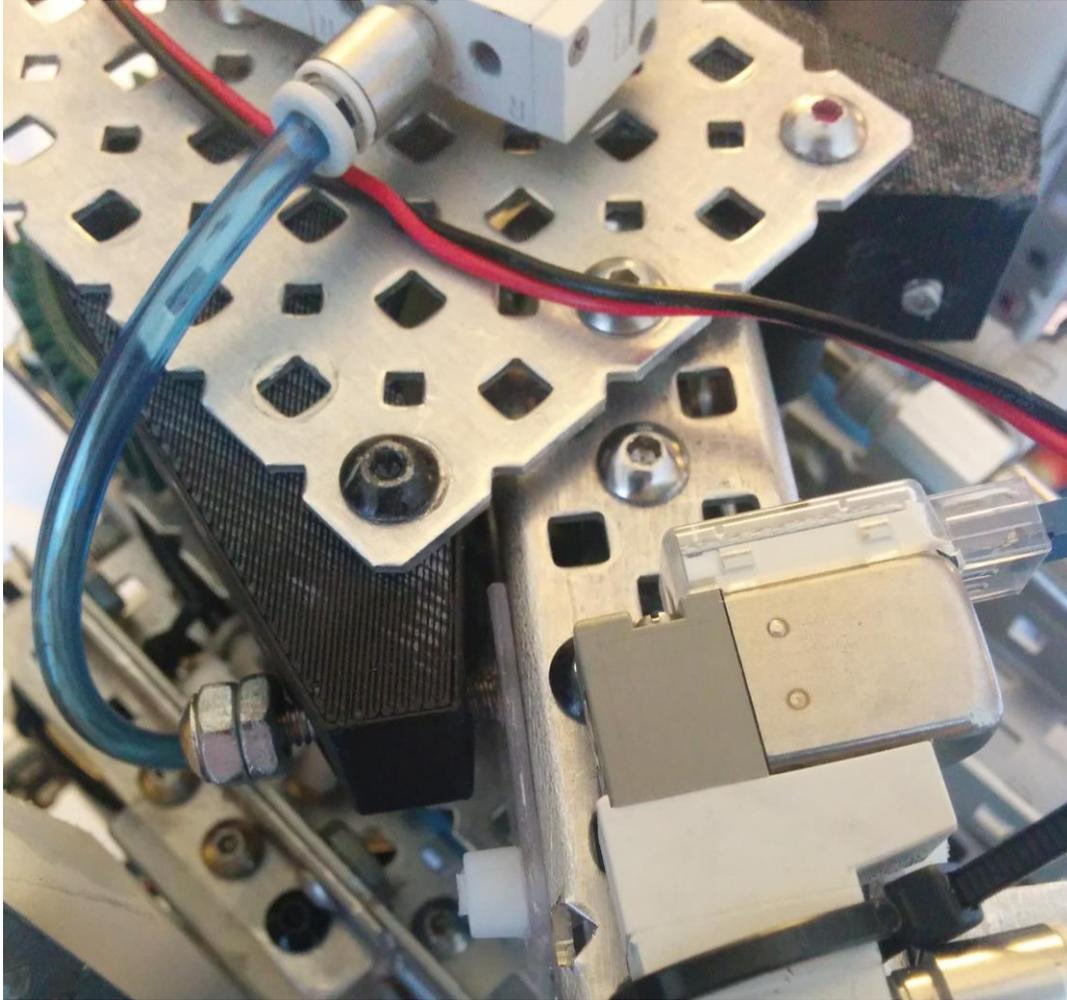
To score cubes McChicken has a single-cube passive hook, which is designed to slide into the cube as the robot drives into it, then lock in place, holding both the position and the angle of the cube. The hook was 3D printed to result in a sturdy intake with the perfect dimensions required to slide in under a cube sitting on the field, and also easily pull away from a cube that has been lowered onto a goal.
