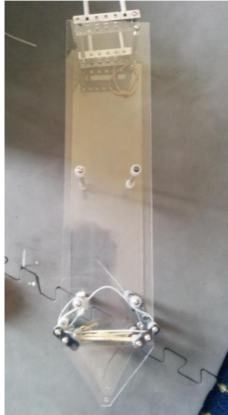
To build this we used 3D printed parts. Both of the allowed large 3D printed parts are used to make the tip of the needle, one of them being a nose cone and the other being the mechanism for the teeth that hold the cubes onto the needle.
