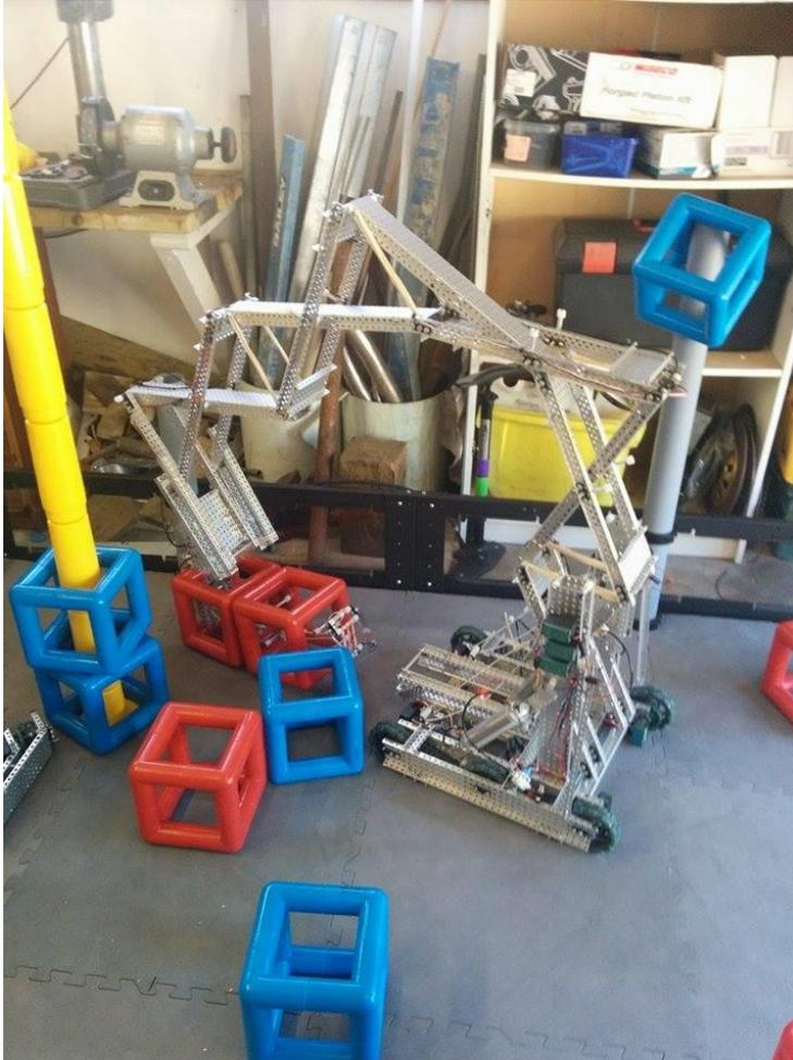
Because of this we instead built a reverse double four bar, powered by 6 motors and driven with a 7:1 reduction. This was a huge improvement in speed, reliability and maximum height compared to the previous scissor lift. The lift is easily able to reach over a full skyrise, and lifts to full height very quickly. Another advantage of the reverse double four bar is that it is linear, the intake does not move back or forward as the arm travels through its range of motion.
