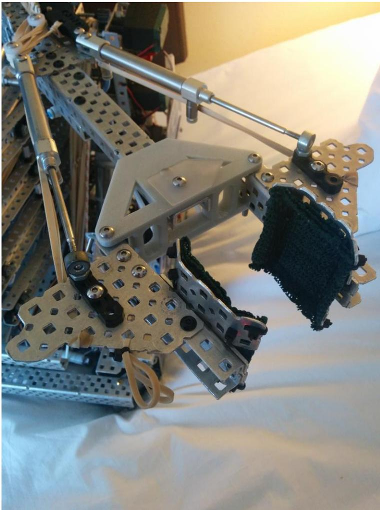
Because Mcchicken was a 15" robot, the swing arm had to fold back to be within size limit. To accomplish this, we used a hinge and latch arrangement, which is rubber banded to unfold when the robot lifts at the beginning of the match.
