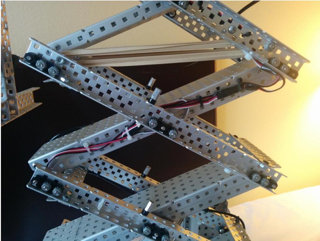
The winch scissor works by having a large driven gear on a tower at the back of the robot. This gear is attached to a spool that uses strings to pull the lift up and down as the winch is wound. The string to raise the lift runs straight off the spool and is connected to the bottom arm, and string to lower the lift is run from the spool, and around a roller at the bottom front of the robot.
