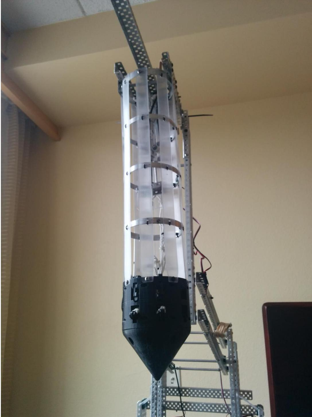
As well as the pneumatic piston to control the movement of the needles teeth, there is an additional piston and another set of teeth which act as a set of locks. The locks are designed to hold the bottom cube down onto the lower section of the needle and stop it from rotating. This helps the needle to align on the post or skyrise when it is lowered. If the cube is locked in place and the post is anywhere within the cube, the point of the needle is guided into the top of the pole.
